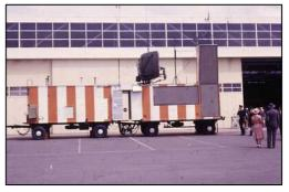
The Butterworth unit was unique, in that it had a third, Australian designed, trailer which contained two rotary frequency converters which allowed the radar to be
