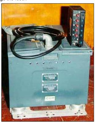
channel 'D' had the ability to be used in 'pipsqueak' mode. Pipsqueak was a homing or DF tone sent from the aircraft to a ground station so the ground station could take bearings on the aircraft. It was useful either for normal DF work or when the aircraft was in trouble and the pilot did not want to stay around to transmit.
