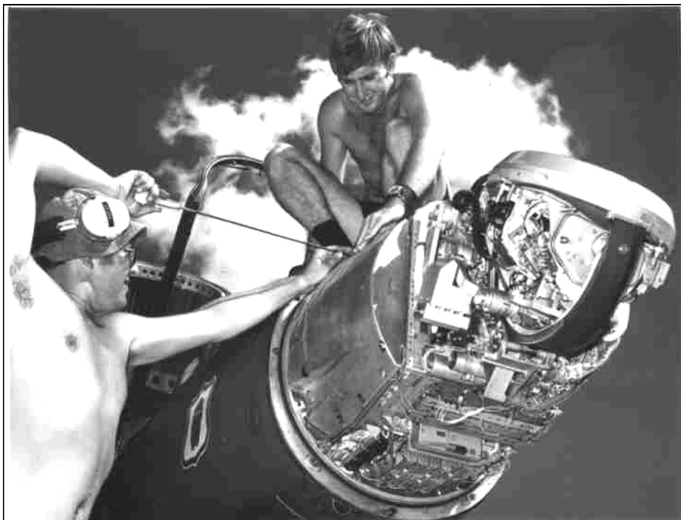
Radio Techs, Ray Farley (standing) and Peter Roberts, working on a 77Sqn Mirage radar during exercise 'Blue Denim' in Darwin 1973.
