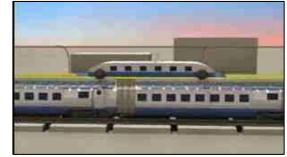
all its passengers, the cabin connector cabin will be moved to the back of the train so that the next batch of outgoing passengers who want to alight at the next station will board the connector cabin at the rear of the train roof. When the train arrives at the next station, it will simply drop the whole connector cabin at the station itself and leave it behind at the station.
