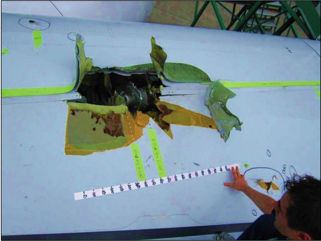
Figure 2: WU-Overall view showing damage to droop nose and D nose (hidden)
