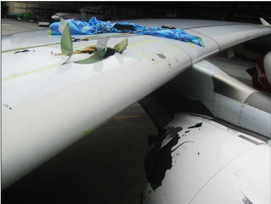
Figure 5: Forward view of engine and subsequent damage for this item.
