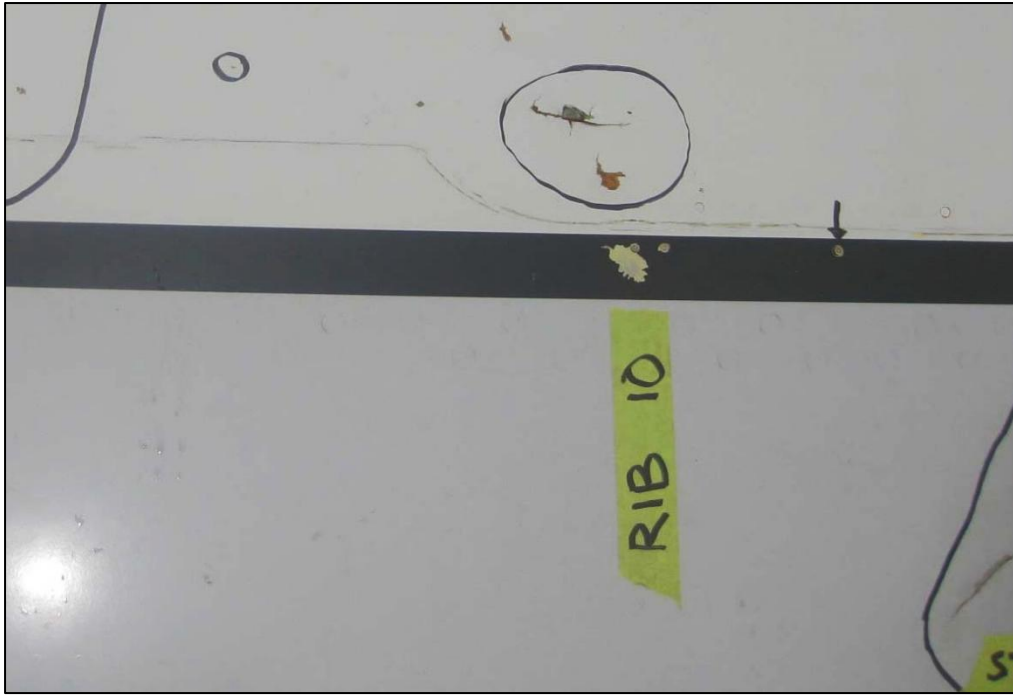
Figure 14: Perforation with metal lodged in structure
