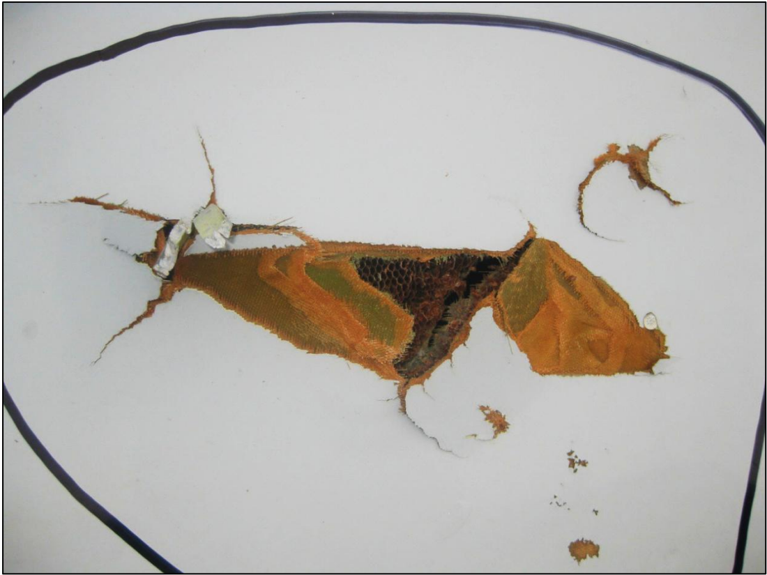
Figure 12: Largest of the 3 skin perforations with metal still lodged in structure
