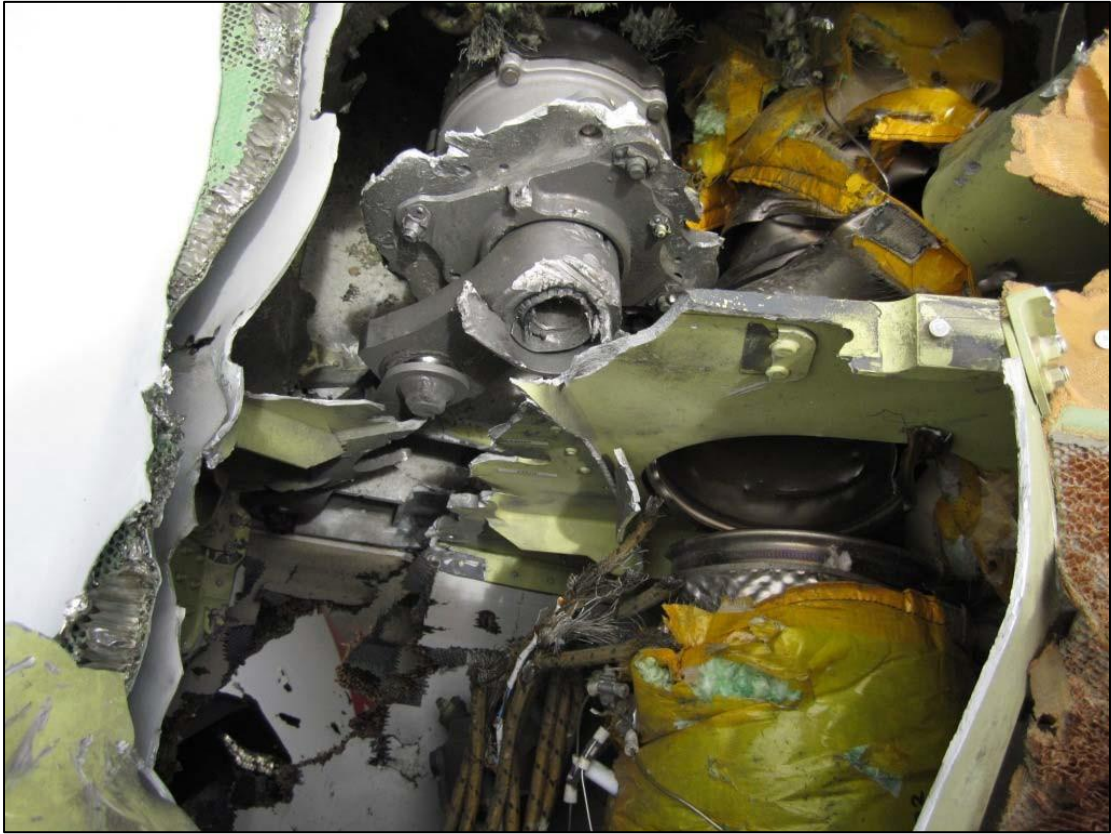
Figure 4; Close up of damage between at leading edge ribs 4 showing droop nose drive motor
