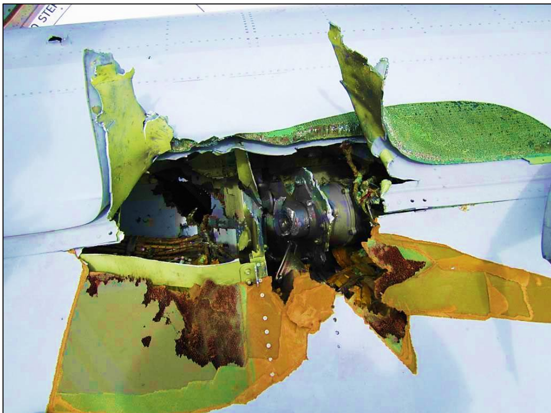
Figure 1: WU-1 Perforation at topskin Rib 12 location
